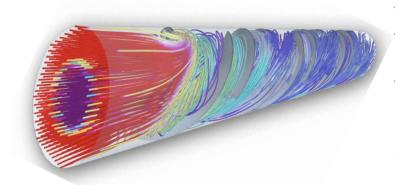
Vortex fluid rotation allows flow across the entire pipe cross-section, which also minimizes sidewall friction. More fluid flows with less energy. Multiple Vortex units compound efficiency and reduce pumping needs by over 40%. Vortex delivers flow assurance across the system.
