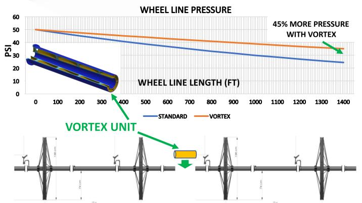
In a 1400' wheel line system **Vortex delivers 45% more pressure** to the end of the line compared to standard systems. Using Vortex units, enough pressure may be maintained **to run more wheel-lines**.
